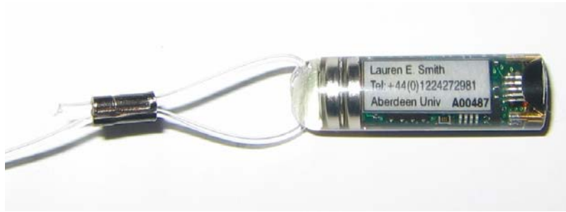
Figure 2. Partial construction of the DST attachment, the DST is threaded onto the monofilament (50 ILB breaking strain) and held in place with a double crimp.
